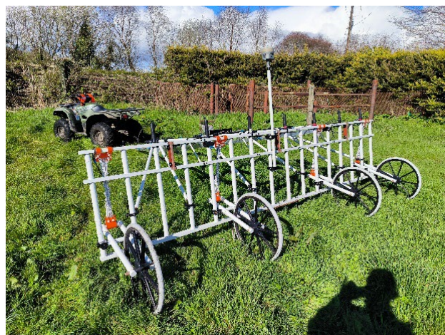
SENSYS MAGNETO® MXV3 modular carrier with 8 SENSYS FGM650/3 sensors spaced at 0.5m intervals
