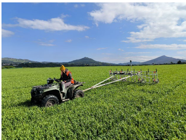
SENSYS MAGNETO® MXV3 modular carrier with 8 SENSYS FGM650/3 sensors spaced at 0.5m intervals
