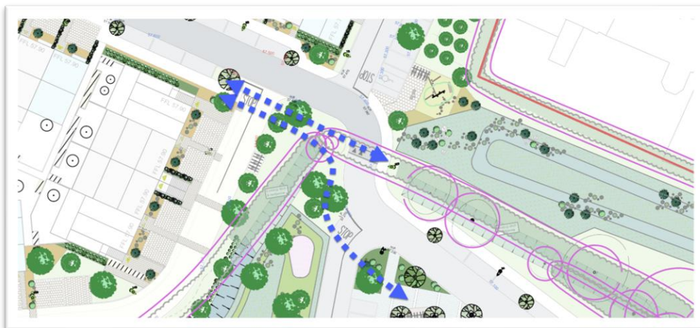
Figure 2.4 – Missing Footpath Links Near Main Pedestrian Access to Captains Hill / Train Station
