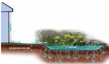
Open attenuation tank, rain-gardens
