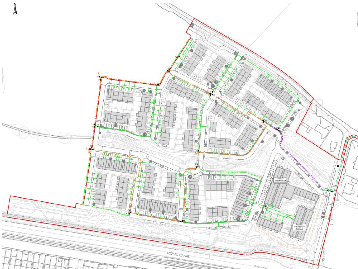
Figure 12 Extract from DOBA drawing C-0401 illustrating the proposed water supply layout (Source: DOBA)
