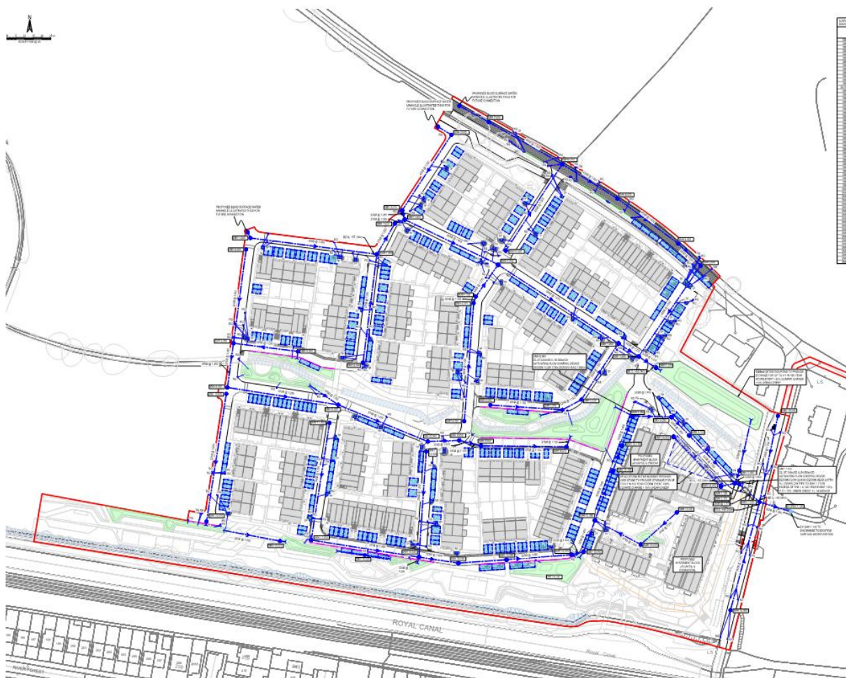
Figure 6 Extract from DOBA drawing C-0200 indicating the proposed SW layout (Source: DOBA)
